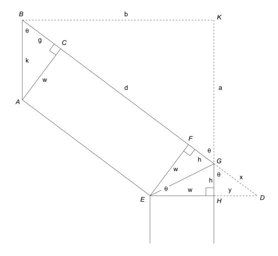
We need to determine the lengths k and h in order to be able to locate vertices A and E as offsets from B and G. We will use similar triangles. The basic triangle is  $\Delta BGK$  with sides
