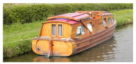
Our canal boat will have a pointed bow and a square stern. The hull will have vertical sides and a flat bottom. The cabin will be a long rectangular box.
