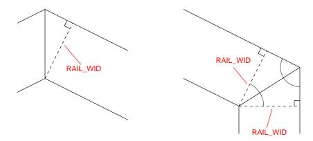
Use similar triangles and the Pythagorean Theorem to calculate the distances from the inside corner of the railing to the outside corner. In each case, that line should bisect the angles formed by the sides of the railing.
